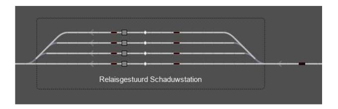
What is now striking is that all detectors in the station have been given a grey frame, unlike the detector in blocks without a relay (see detector on the right for the shadow station). This indicates that these detectors are part of a relay-controlled block and the block is switched off. Just click as a test on any relay:
