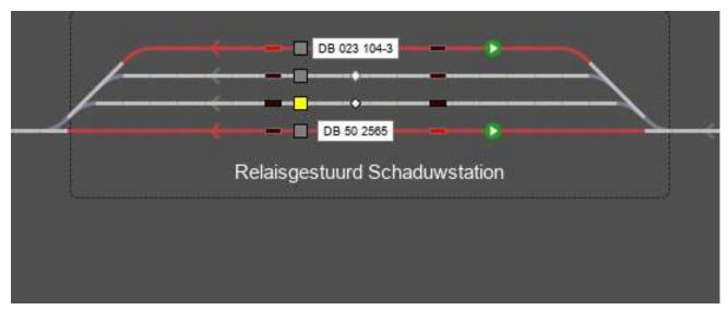
Here you can see that two trains are already present, that the third track is active without the detectors reporting. Which makes sense, because the relay circuit only allows the detectors to see the sections that are connected by the relay to the block output. In this case the third track seen from above.
