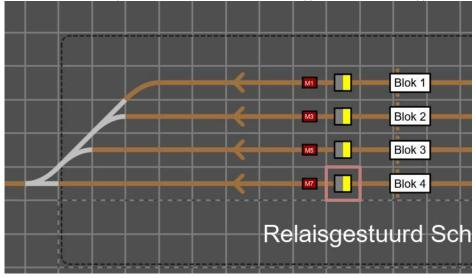
Each relay is given its own unique name, for example R1, R2, R3 and R4. While setting up the relay in the OCConfig, an address was issued for each relay. We assign this address to the correct relay.
