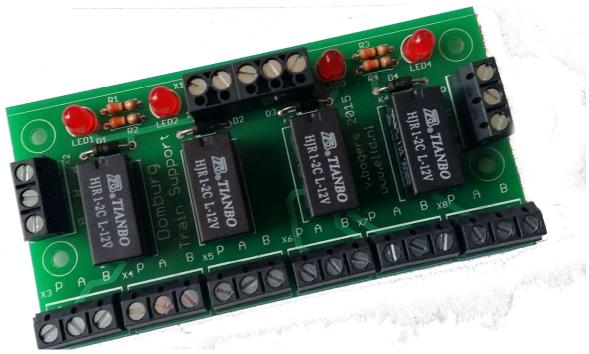
The HPP4 relay board has a simple but effective operation. The base revolves around the 4 relays. Each relay is equipped with 2 changeover contacts which switch as soon as the relay is energized.
