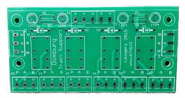
K1 has the screw terminals X2 and X3 K2 has the screw terminals X4 and X5 K3 has the screw terminals X6 and X7 K4 has the screw terminals X8 and X9
