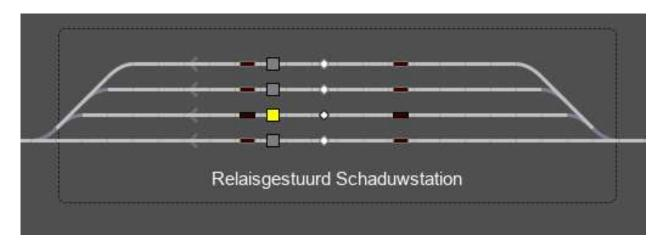
You can now see that the block is switched on because in addition to the status of the relay being changed, the detectors have also become active.
