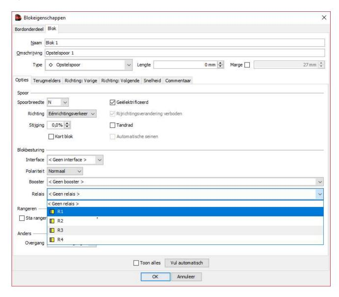
At "Relay", select the relay that is drawn in that block. Then click on "Fill automatically" and now repeat this for all blocks. When you have done this, leave the switchboard editor and go to the regular screen. You will then see this:
