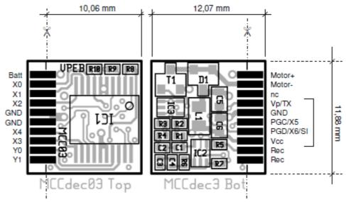
The connection diagram of MCCdecO3 is almost equal to the one of MCCdecO2. Just mark that MCCdecO3 is one connection pad narrower than MCCdecO2 (so in total 20 in stead of 22). At MCCdecO2, the Motor-minus is located at the corner, at MCCdecO3 that connection has "jumped over the Motor-plus". That pad was unused on MCCdecO2. Further the double Vbat(+) is degraded to a single one.
