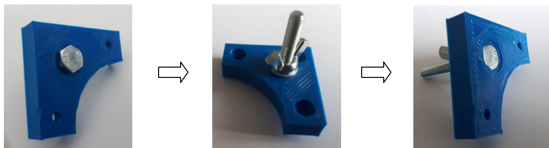
Figure 2: Install hexagon bolt in base block
